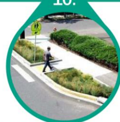
Planted curb with pedestrian gaps
